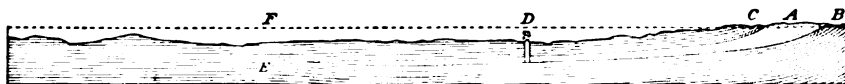
FIG. 2.—Section illustrating thinning out of porous water-bearing bed A , inclosed between impervious beds B , C , thus furnishing conditions for artesian well at D , but not at E .
